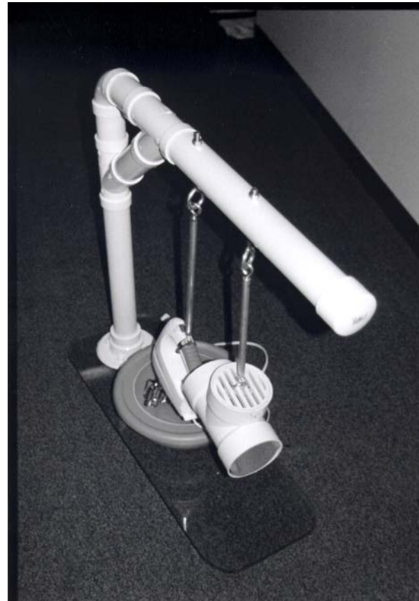
Figure 13.11. Top Left Side View of Support and Guide for Use of an electric mixer.
