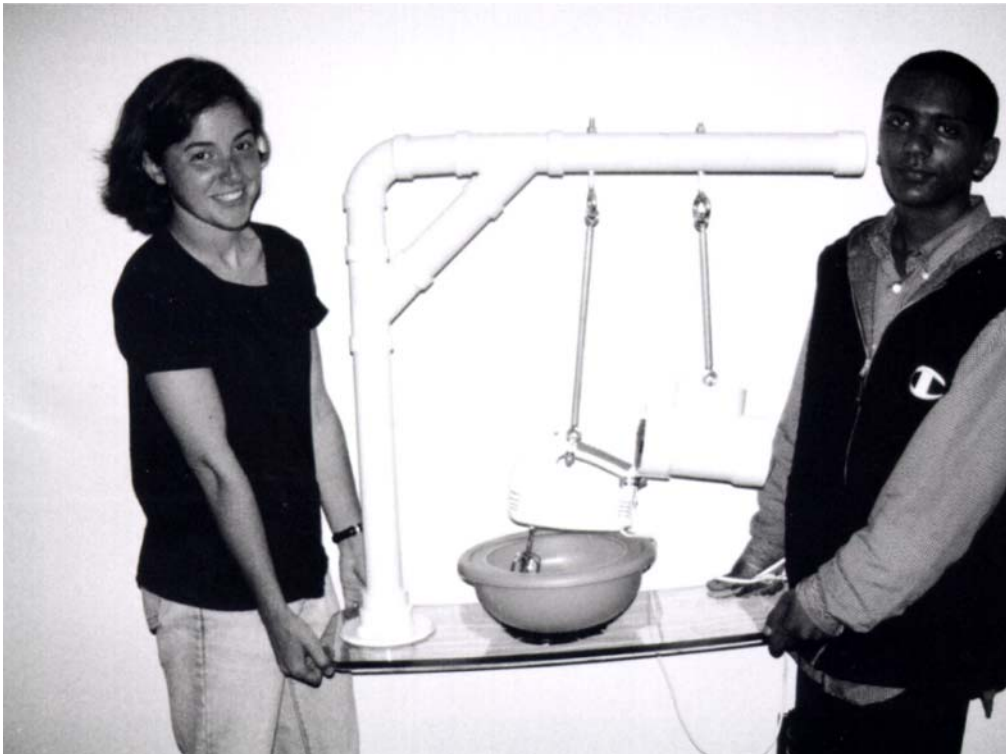
Figure 13.12. Front View of Support and Guide for Use of an electric mixer.
