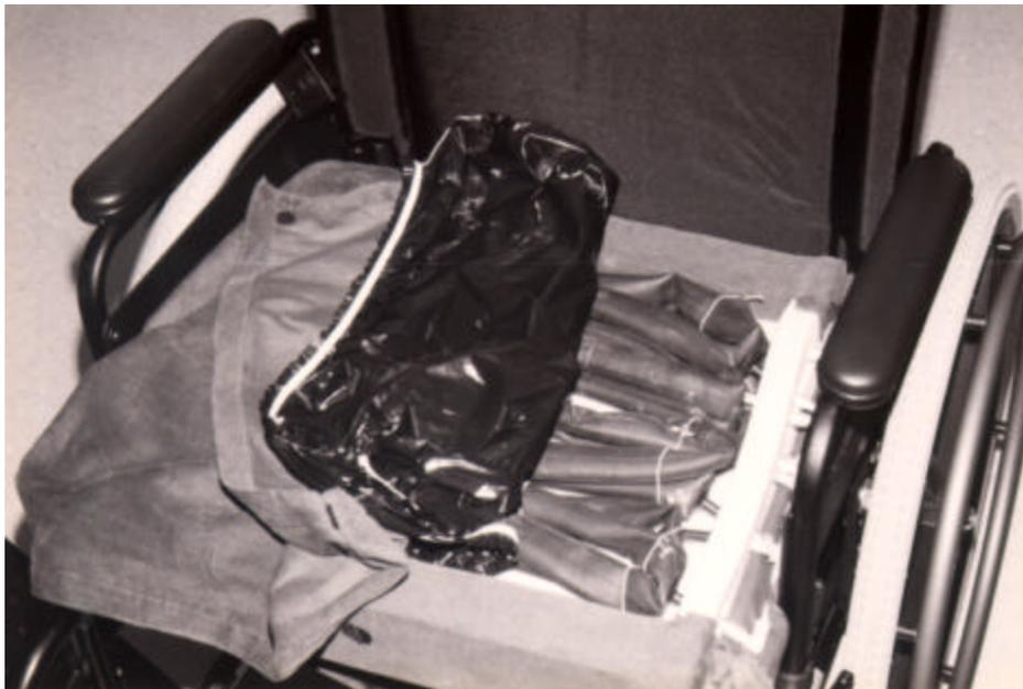
Figure 8.6. - Air Tubes Imbedded in Cushion.
