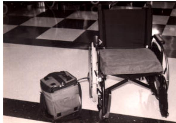
Figure 8.5 - Active Pressure Relief Cushion With Control Box.
