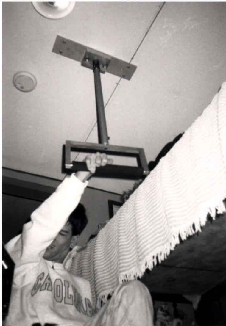
Figure 6.8. Bed-to-Wheelchair Transfer Apparatus.
