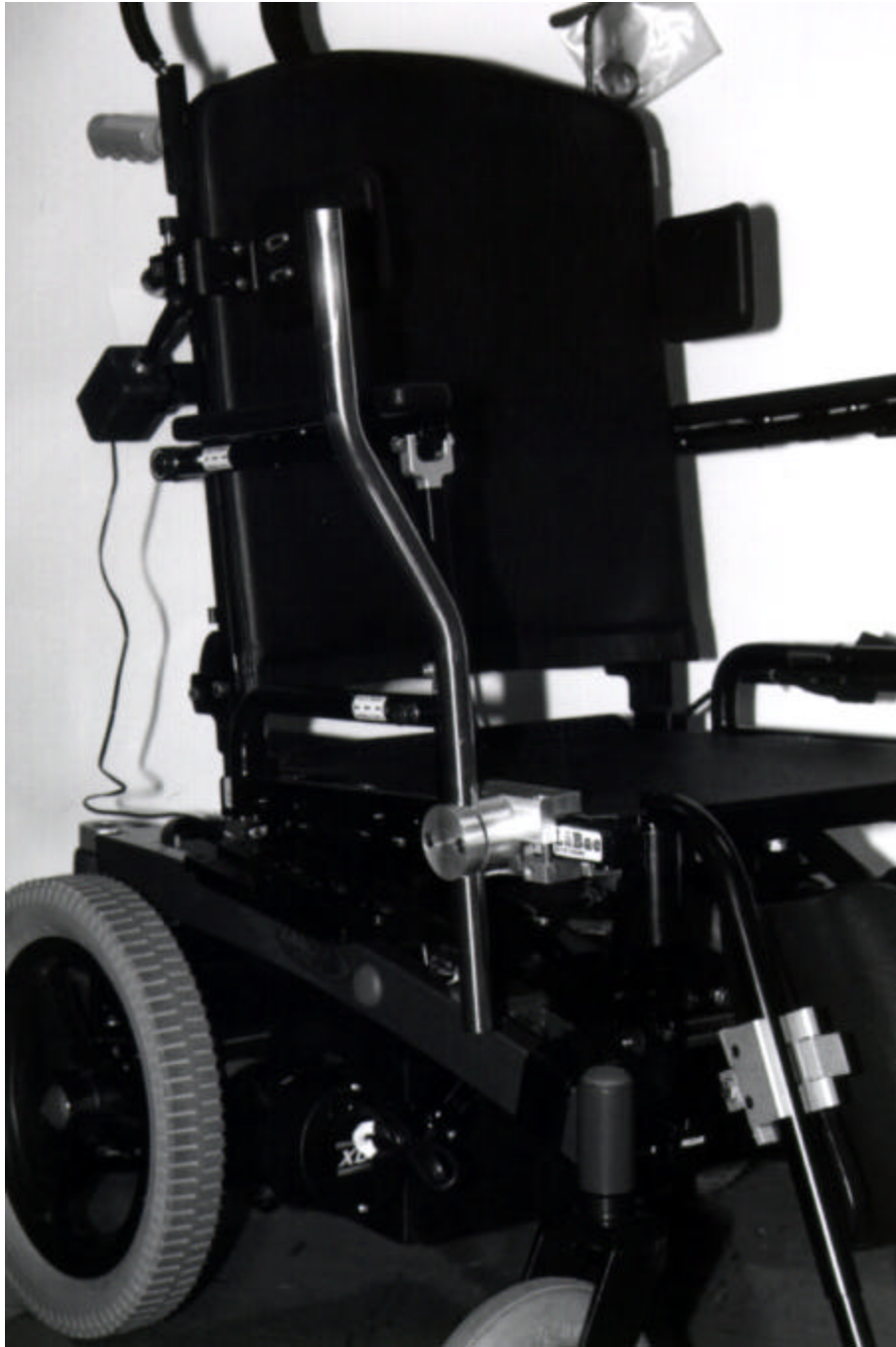
Figure 19.1. Wheelchair Mounting Clamp for a Laptop Computer.
