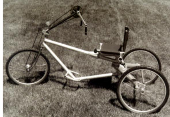
Figure 18.7. Three-Wheeled Hand Powered Cycle.
