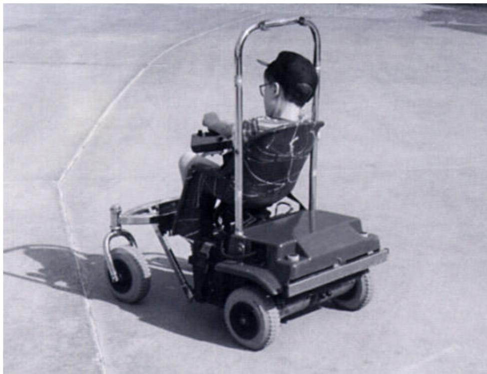
Figure 18.5. Child's Joystick-Controlled Go-Cart
