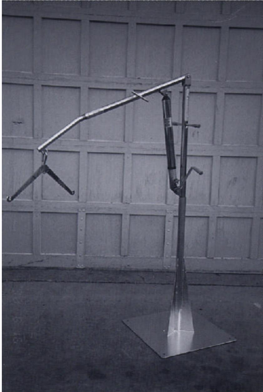
Figure 18.2. Trailer Mounted Personal Lift Transfer System.
