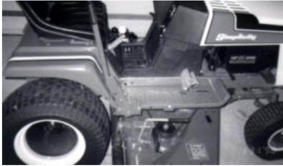
Figure 17.3. Clutch Pedal Before Modification.
