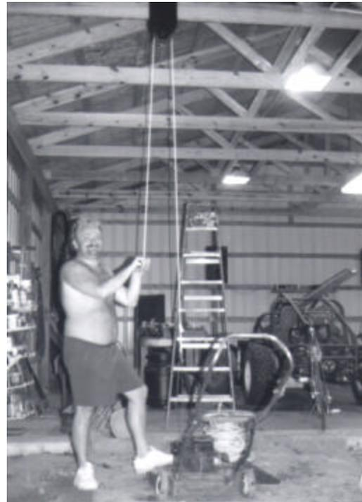
Figure 17.15. Assistive Lawn Mower Starter.
