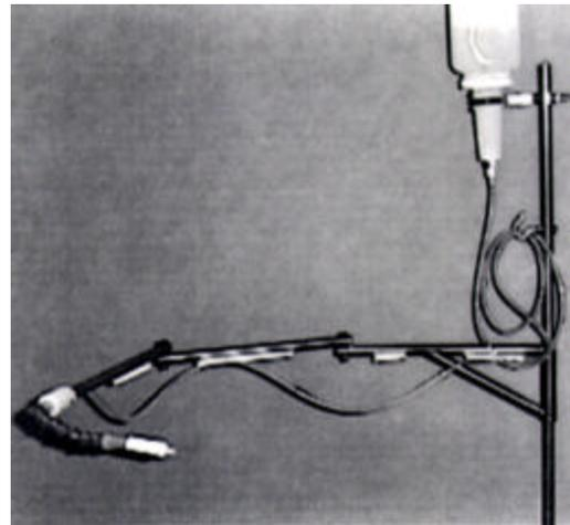
Figure 17.13. Drinking Unit Mounted on a Hospital Bedpost with Arm Extended.
