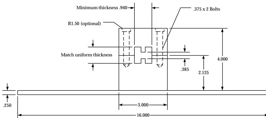
Figure 17.19. Schematic Showing the Machining of the Fixation Blocks Allowing Insertion of the Machined Handle (Dimensions in Inches).
