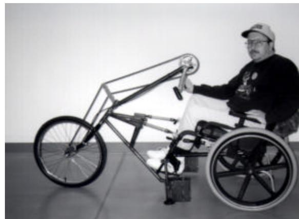
Figure 17.24. Tricycle in Use by a Client with Quadriplegia.
