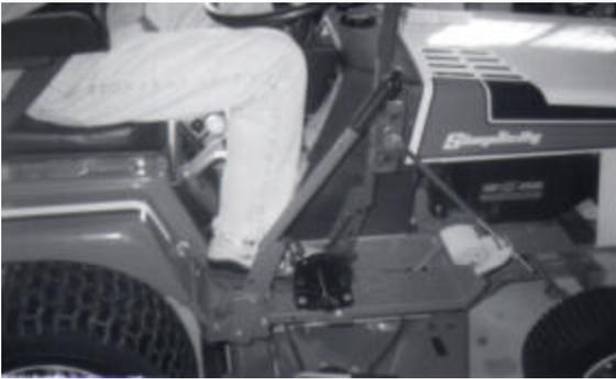
Figure 17.8. Clutch Lever Arm Assembly Fully Installed
