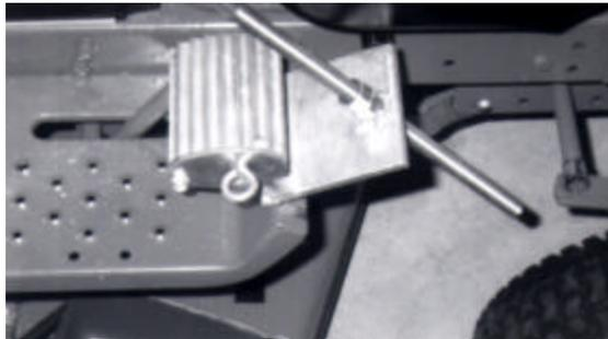
Figure 17.4. Clutch Pedal After Modification.
