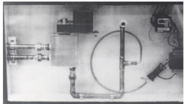
Figure 17.26. Temperature Control Shower Unit. The System Includes: (1) Motor; (2) Mixing Valve, (3) Thermocouple, (4) PID Controller, (5) Transformer, (6) Hot Supply Line, (7) Cold Supply Line.
