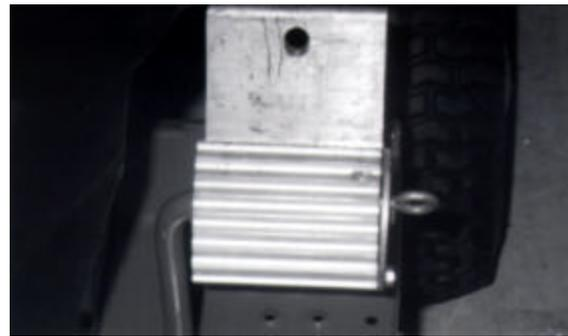
Figure 17.6. Modified Clutch Pedal Mounted On Clutch Bar After Phase 1 Installation.
