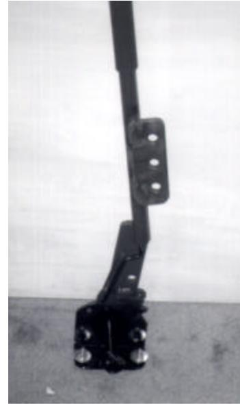
Figure 17.1. Modified Clutch Lever Arm.
