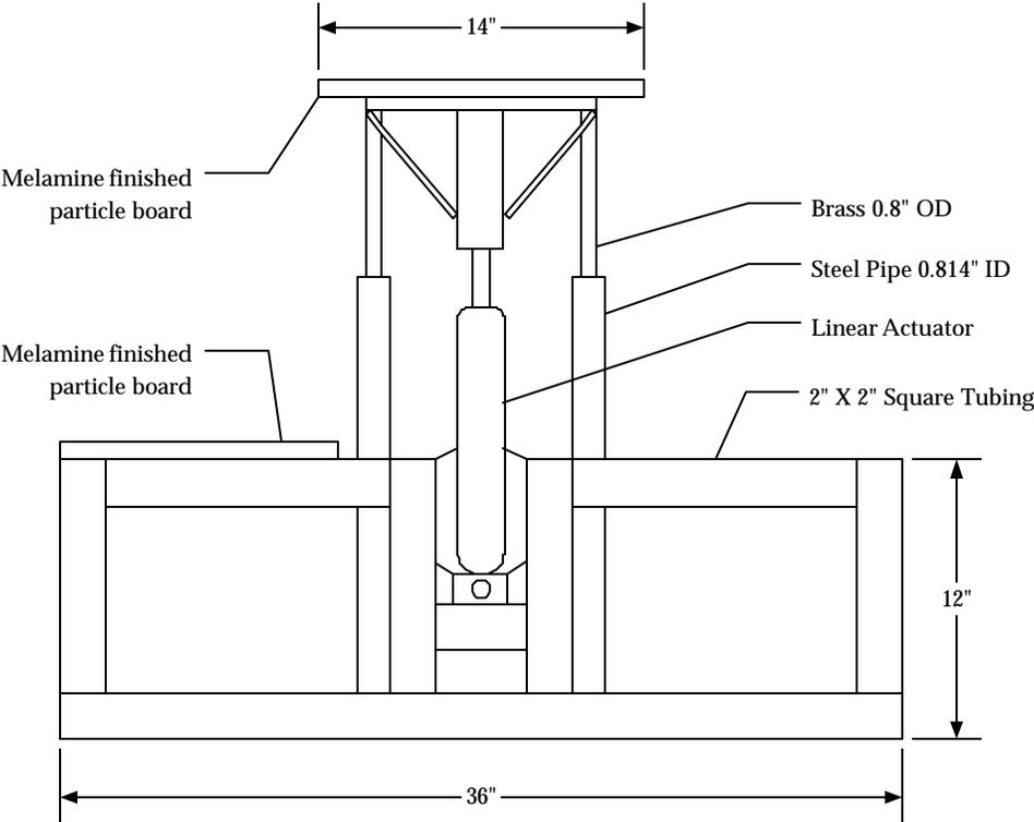
Figure 16.4. Diagram of Computer Workstation.
