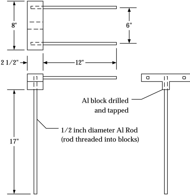
Figure 16.8. Diagram of Laptop Support.
