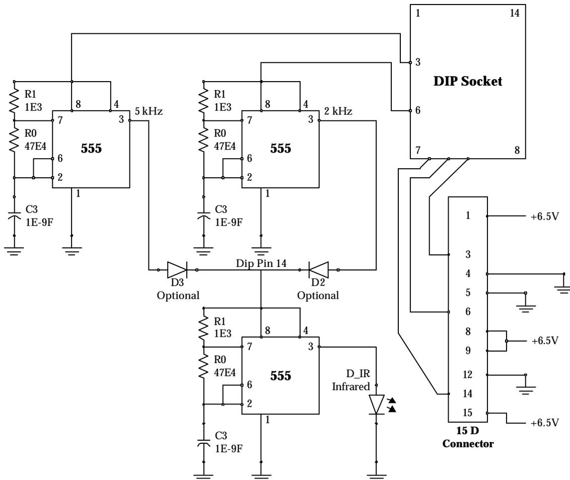
Figure 14.1. Schematic of a Simple, Three-Command IR transmitter.
