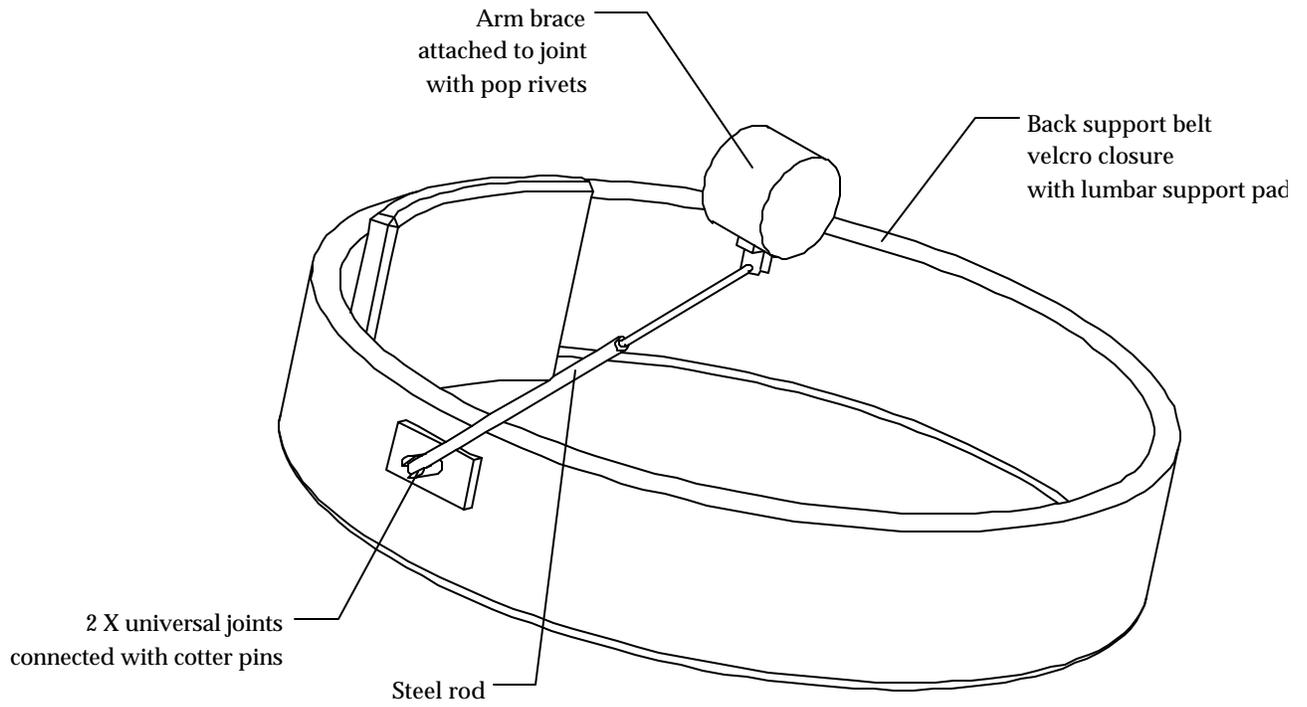
Figure 14.5. Arm Brace Assembly.
