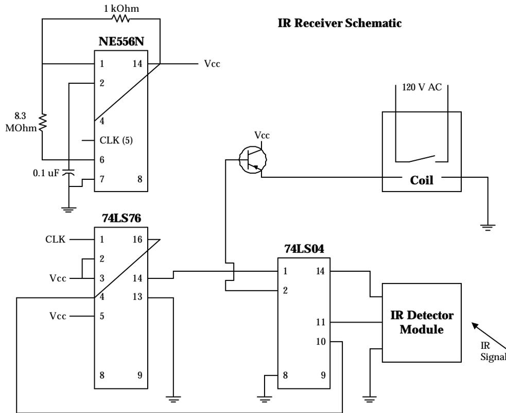
Figure 14.2. Electric Wiring Diagram of a Toggling Relay Circuit that Responds to IR Input.
