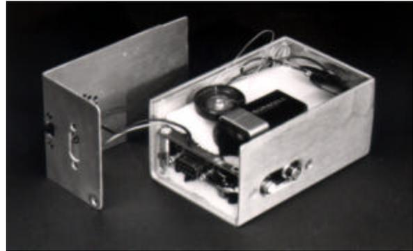
Figure 12.1. Portable Speech Analyzer Internal View.
