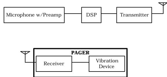
Figure 12.2. Block Diagram of the Wireless Infant Monitoring Device.
