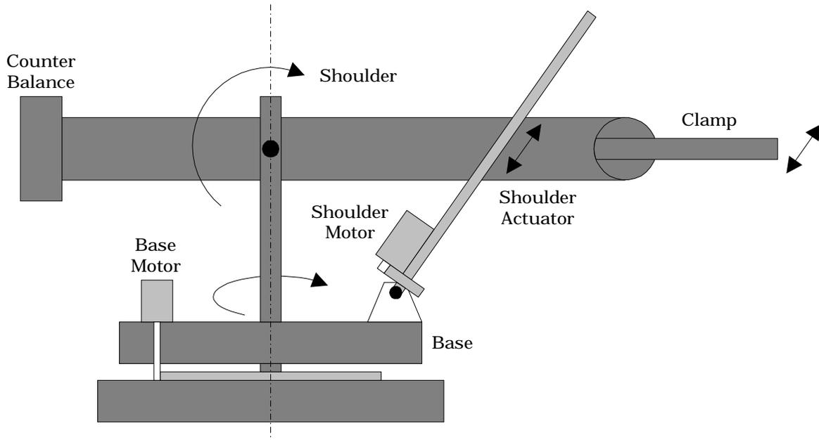
Figure 9.3. Mechanical Configuration of the Motorized Clamp.
