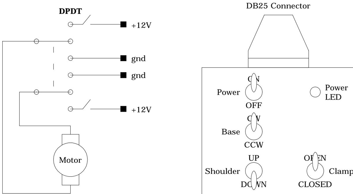
Figure 9.4. Electrical Configuration of the Motorized Clamp. Each of the three motors can be driven forward or backwards. To prevent overextending a joint, sensors are used to shut off power to the motor if driven too far.
