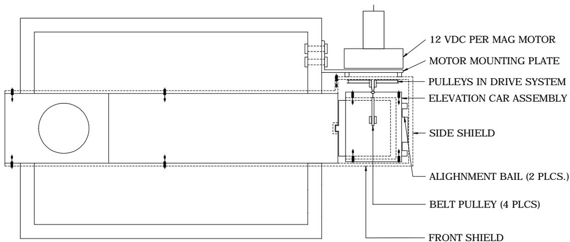
Figure 19.6. Schematic of Drive System: Top View.
