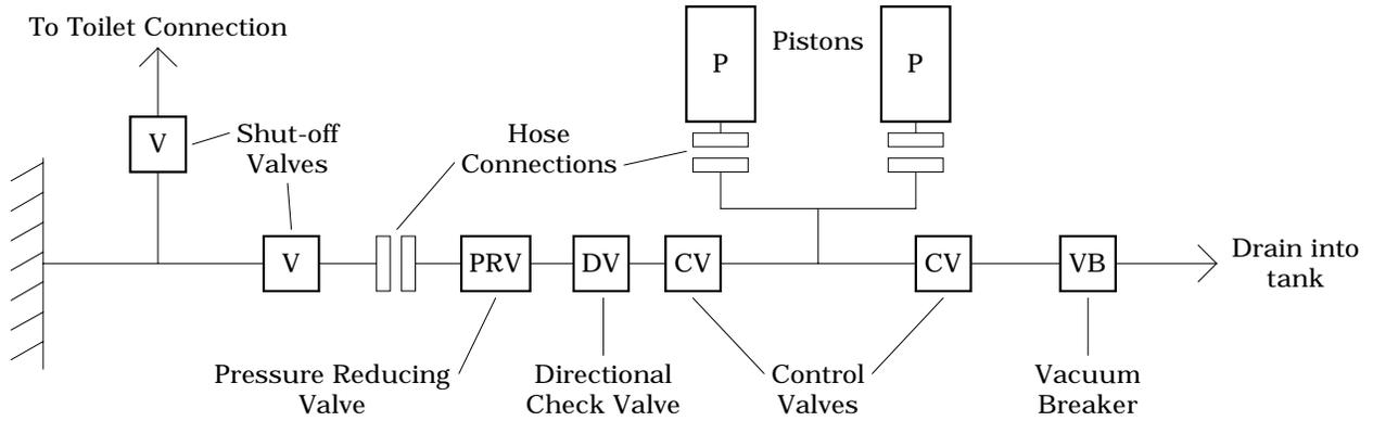
Figure 19.4. Plumbing Diagram.
