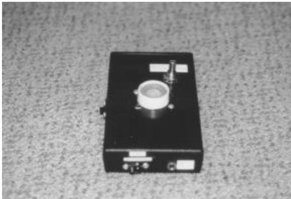
Figure 7.10. The Motion Sensor Switch.
