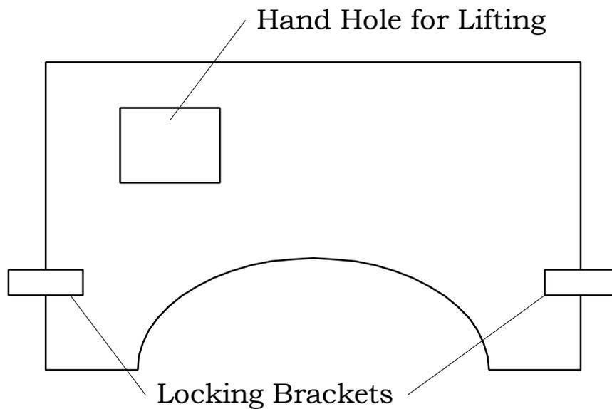
Figure 6.8. Line Drawing of Lap Table Layout.
