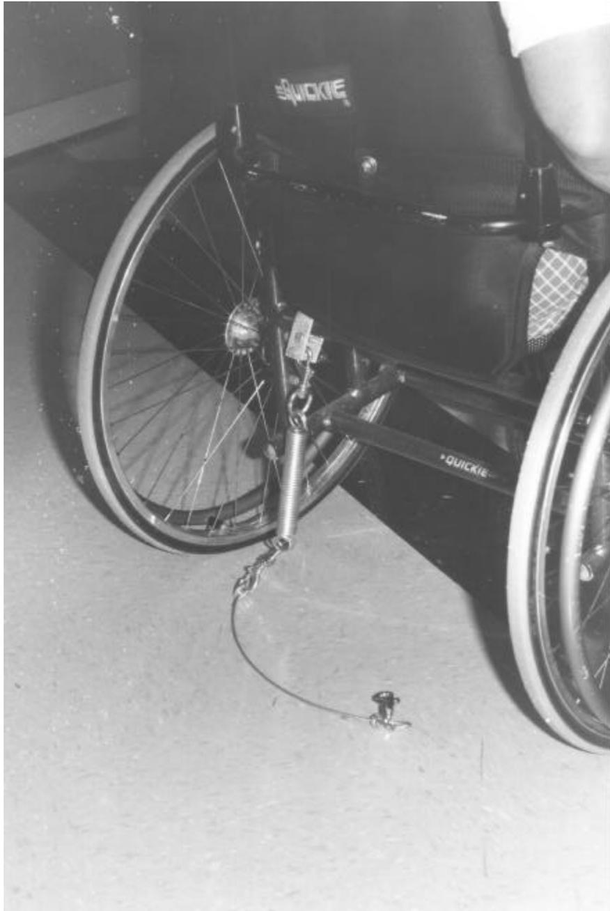
Figure 6.5. The Attachment of the Connector and Latching Spring to the Wheelchair.
