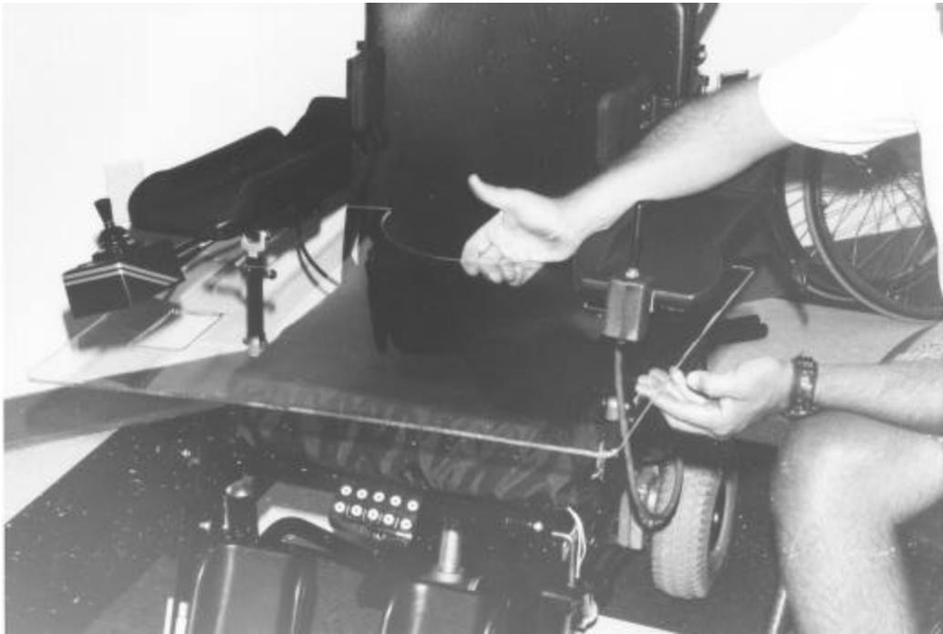
Figure 6.9. The Quad-Friendly Lap Table as it Fits on a Wheelchair.
