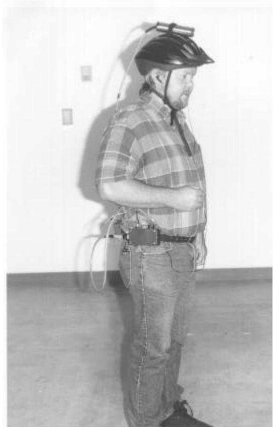
Figure 6.1 Ultrasonic Ranging Device.
