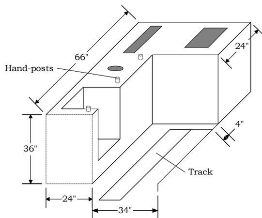
Figure 2.6. View of Wheelchair Operable Checkstand.
