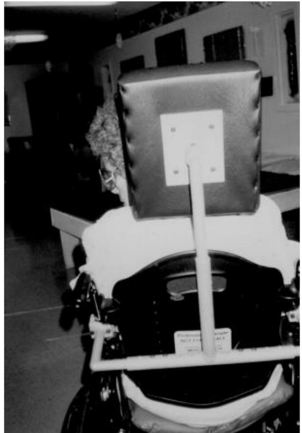
Figure 2.5. Back view of the Detachable Headrest.
