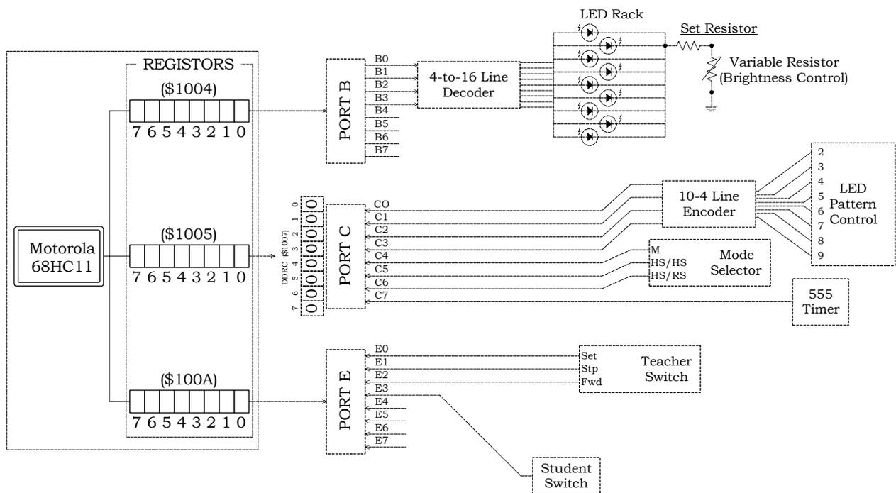
Figure 13.4. PinCorrection for the M otorola M icroprocessor.
