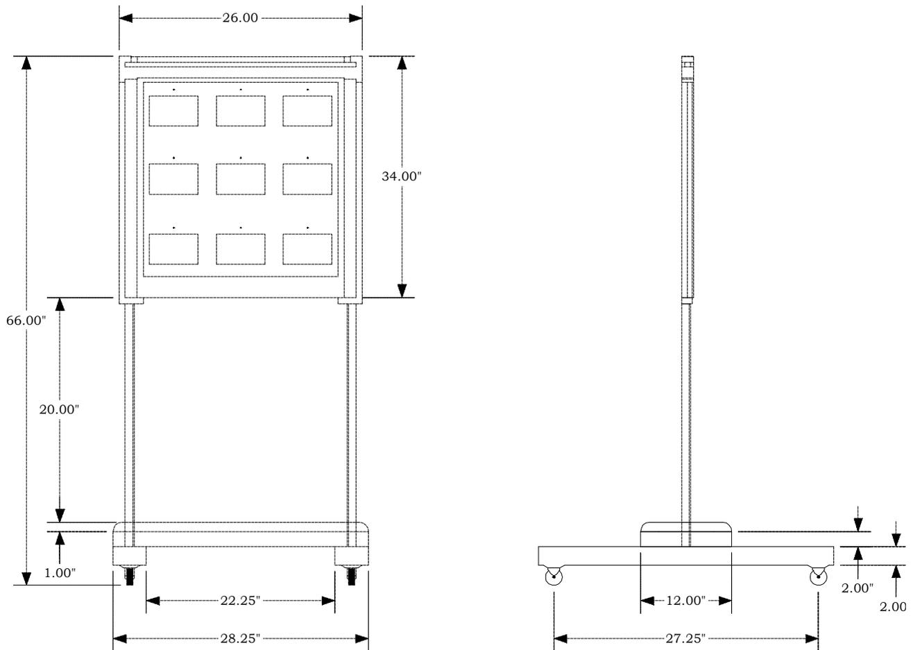
Figure 13.2 Schematic Drawing of the Electronic Eye Gaze Trainer.
