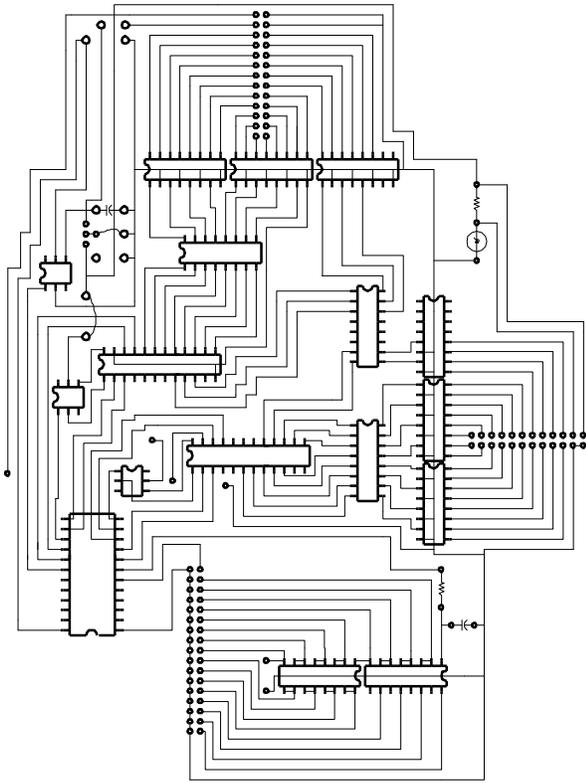
Figure 13.12. Printed Circuit Board Layout of the Environmental Control Unit.
