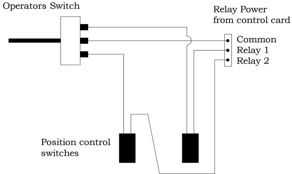
Figure 13.5. Wiring Diagram for Operators Switch and Position Switches.
