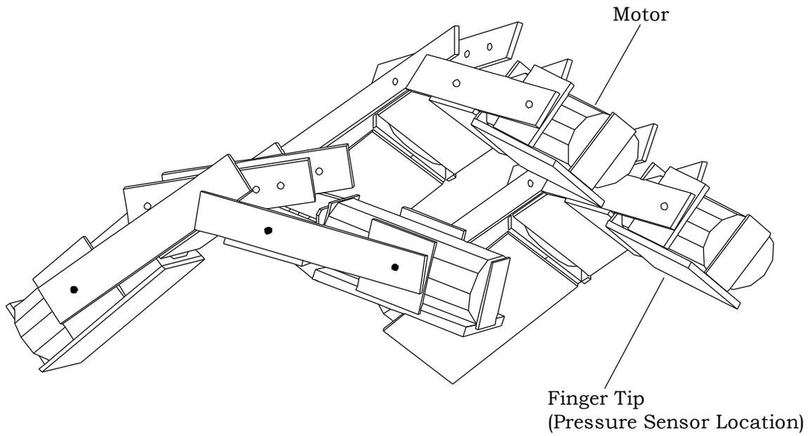
Figure 13.13. Prosthetic Hand with Electric Motors and Force and Position Sensors
