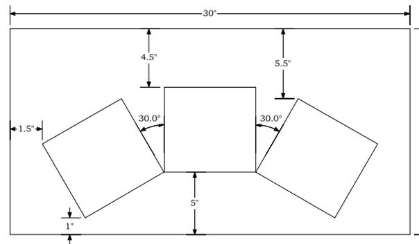
Figure 13.8. Top View of Bin Placement.
