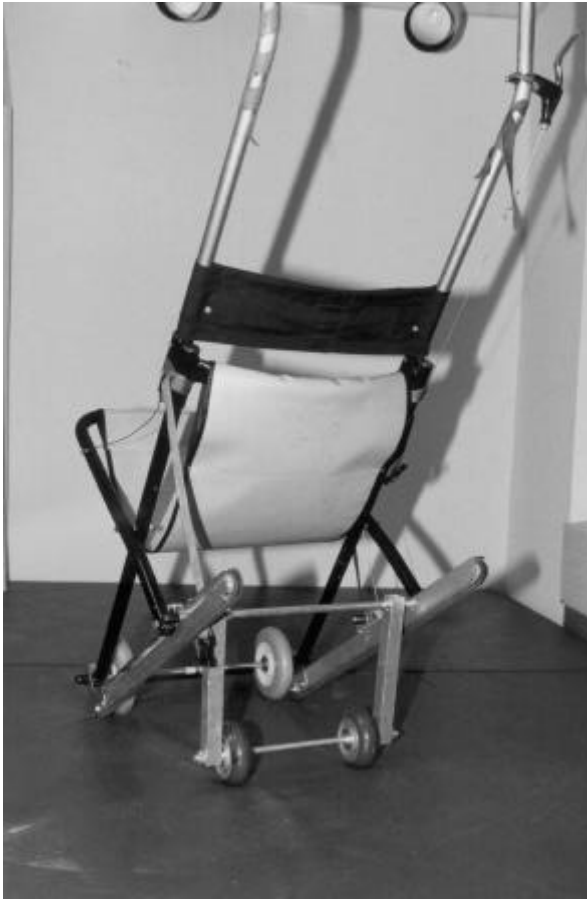
Figure 12.6. Use of Evac Chair with Adaptation to Facilitate Fast Transport on the chair. The two square tubes also rotate about the existing round bar when they are released. After the square tubes and wheels are released, they lock vertically into place by means of a half-moon
