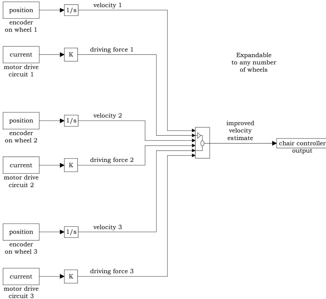
Figure 11.6. Control System Design
