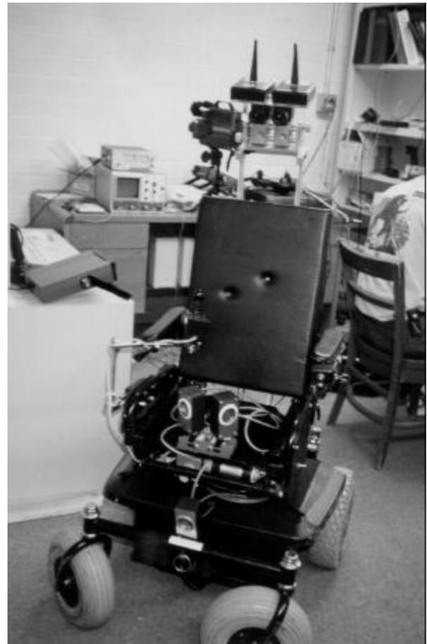
Figure 11.7. Autonomous Wheelchair Cameras and Mounts.
