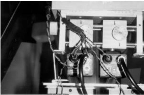
Figure 11.8. Close-Up Photograph of the Autonomous Wheelchair Camera and Mounts.
