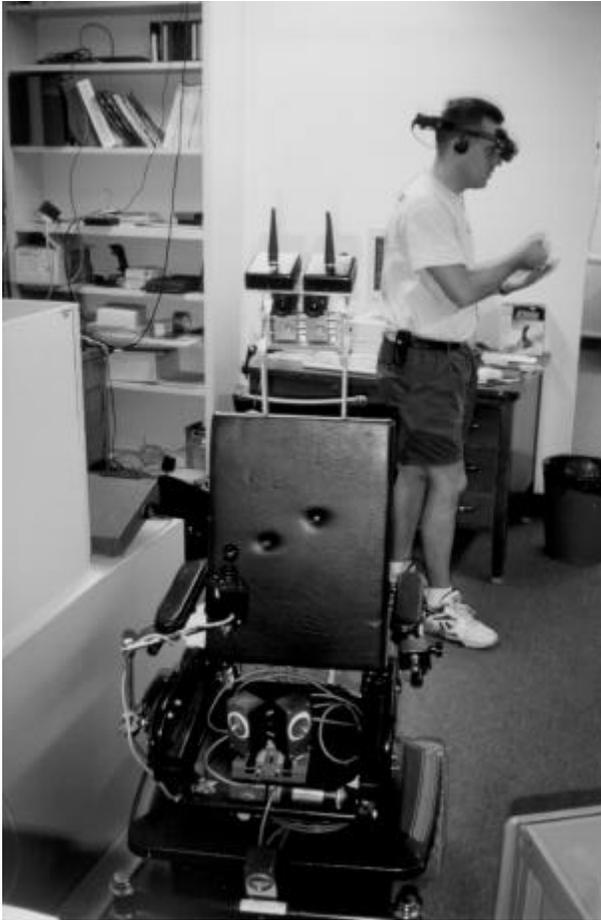
Figure 11.2. Short-Range Autonomous Wheelchair.
