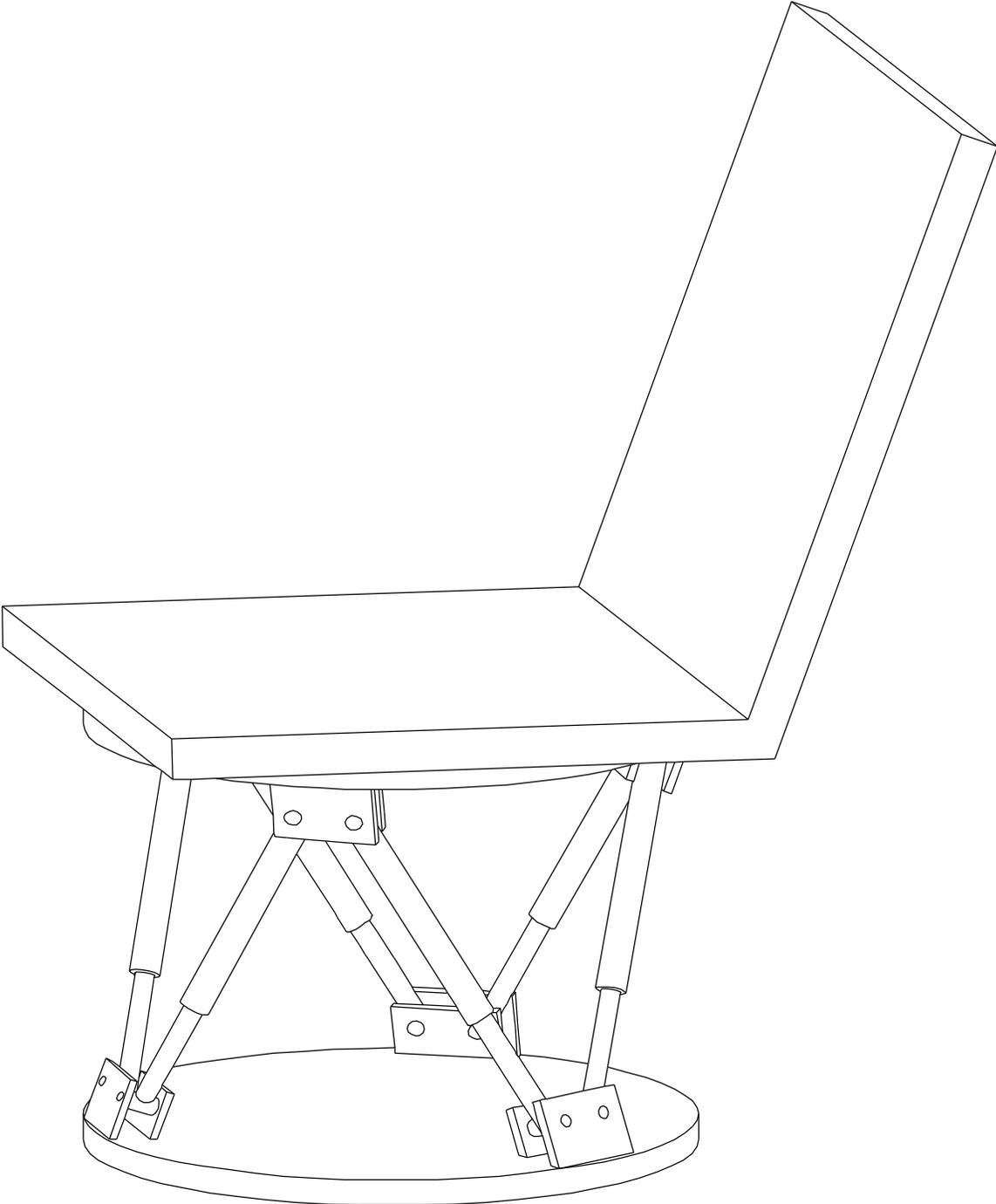
Figure 11.9. Diagram of the Motion Feedback Platform for Virtual Presence Control of the Power Chair.
