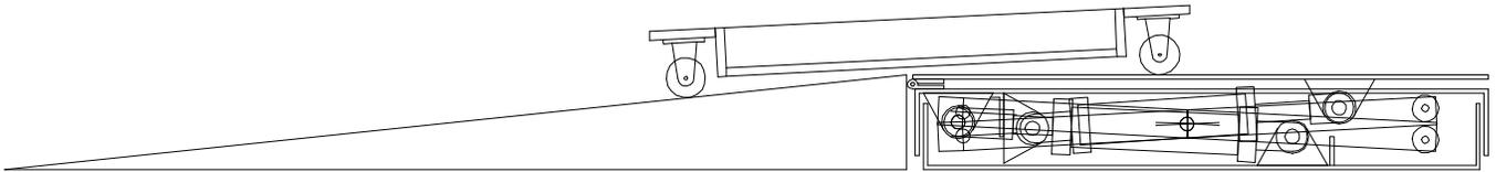
Figure 10.5. Detail Cart Clearance Over Ramp.
