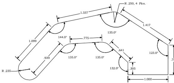
Figure 10.8. Geometric Details Of A Finger Profile.
