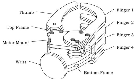
Figure 10.6. Prosthetic Hand in a Pincher Grip
