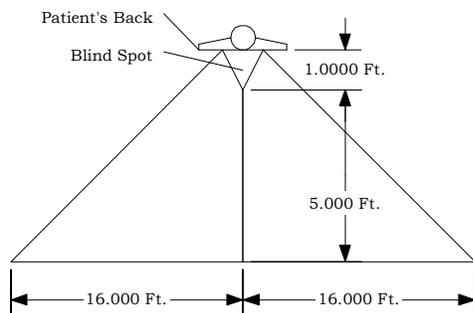
Figure 10.11. Rearward Viewing Area With Convex Mirrors.
