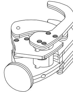
Figure 10.7. Prosthetic Hand When Fully Closed.
