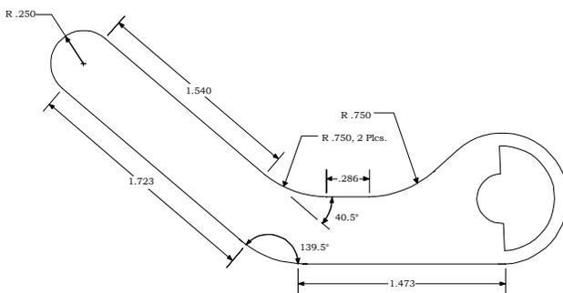
Figure 10.9. Geometric Details Of Thumb.
