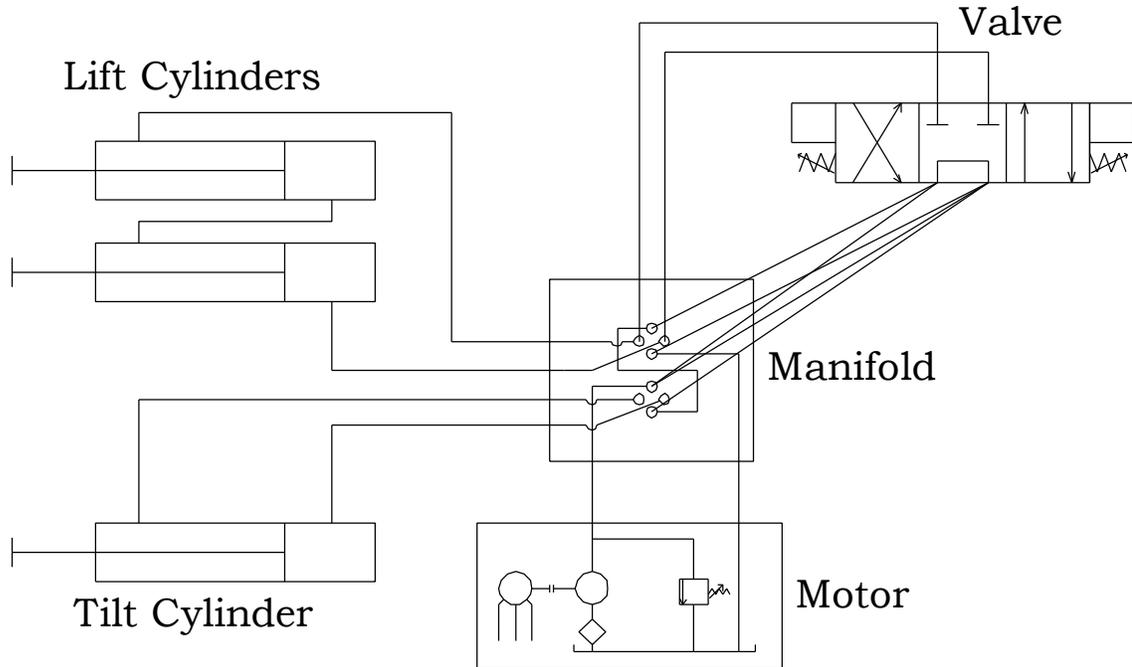
Figure 10.4. Flow Diagram Of The Hydraulic System .
