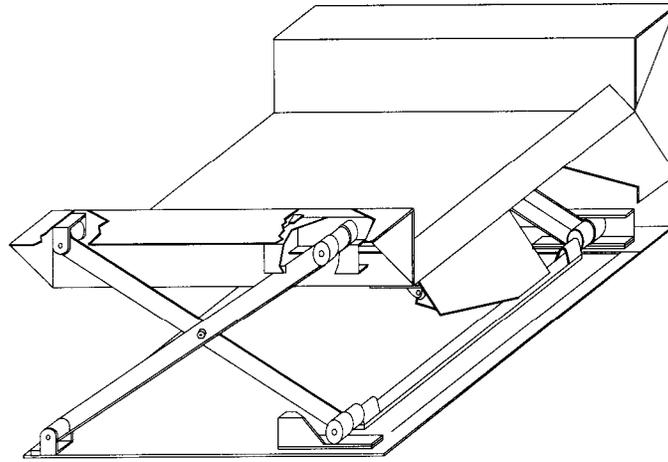
Figure 5.4. Three-dimensional view of lift mechanism minus the lifting source.
