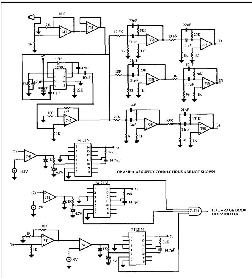
Figure 19.2. Schematic for the Voice Activated Door Opener.
