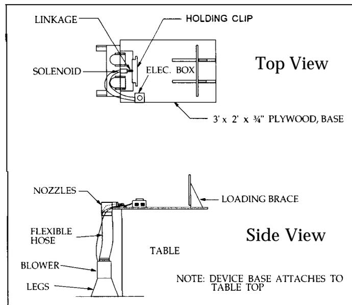
Figure 15.2. Drawing of Paper Product Loading Aid.
