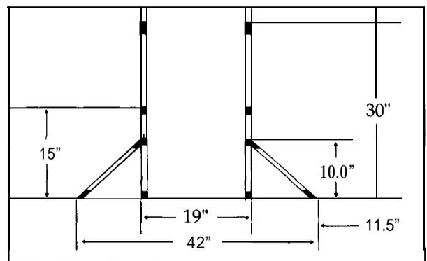
Figure 13.3. Front View of Handrails.
