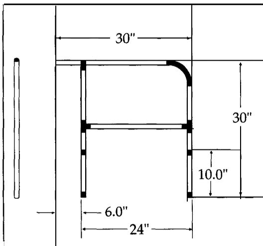
Figure 13.2. Side View of Handrails.
