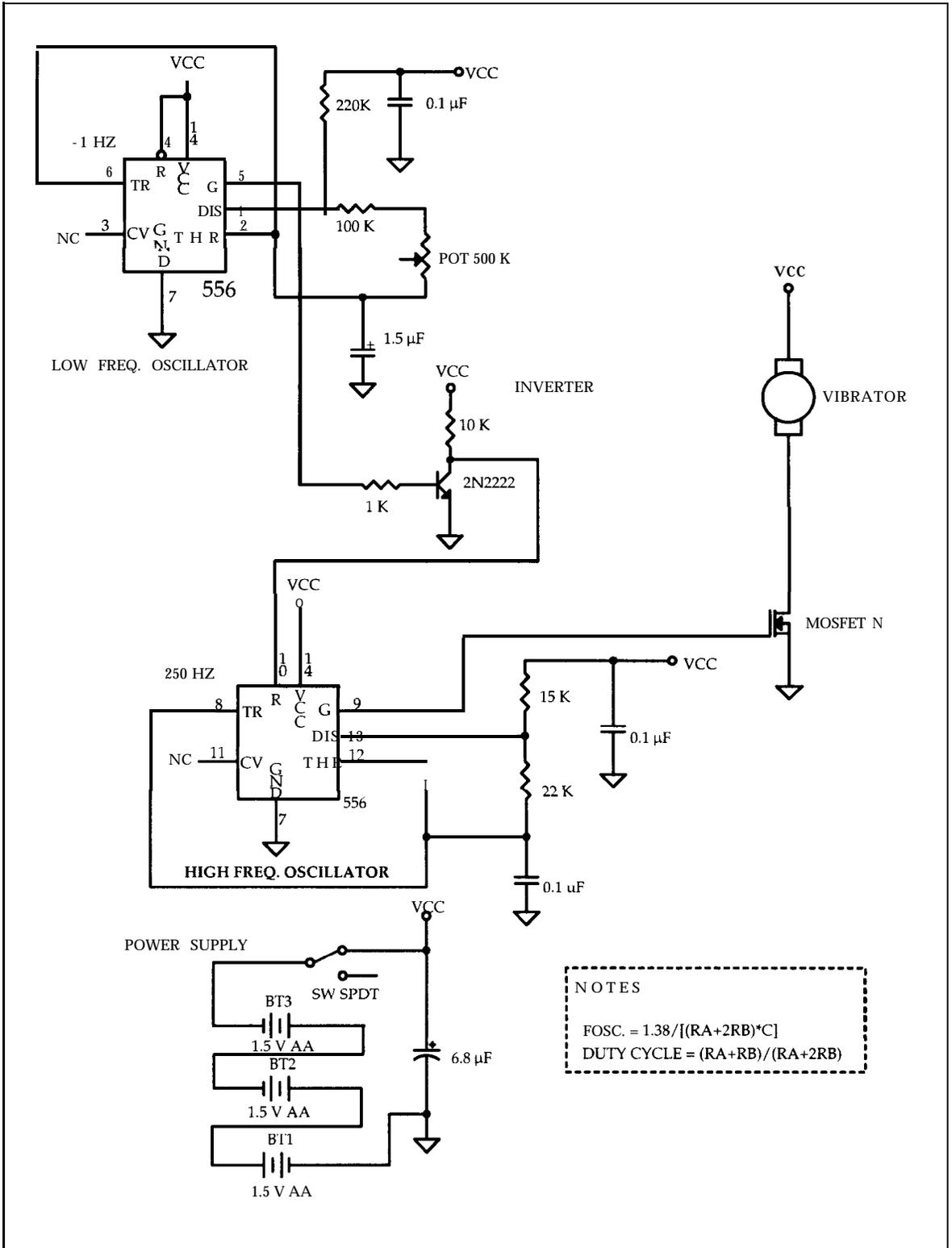
Figure 13.9. Schematic of Tactile Vibrator
