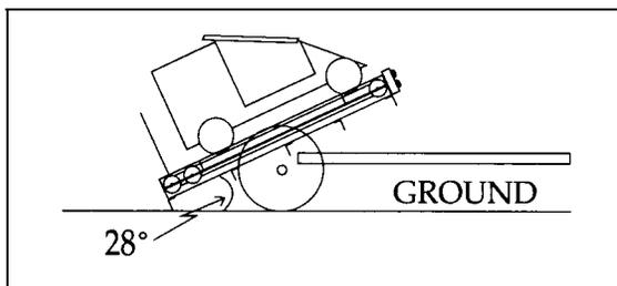
Figure 13.5. Trailer Fully Tilted.
