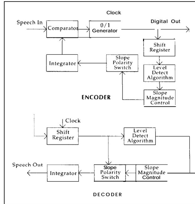
Figure 3.3. Block diagram of CVSD encoder and decoder.
