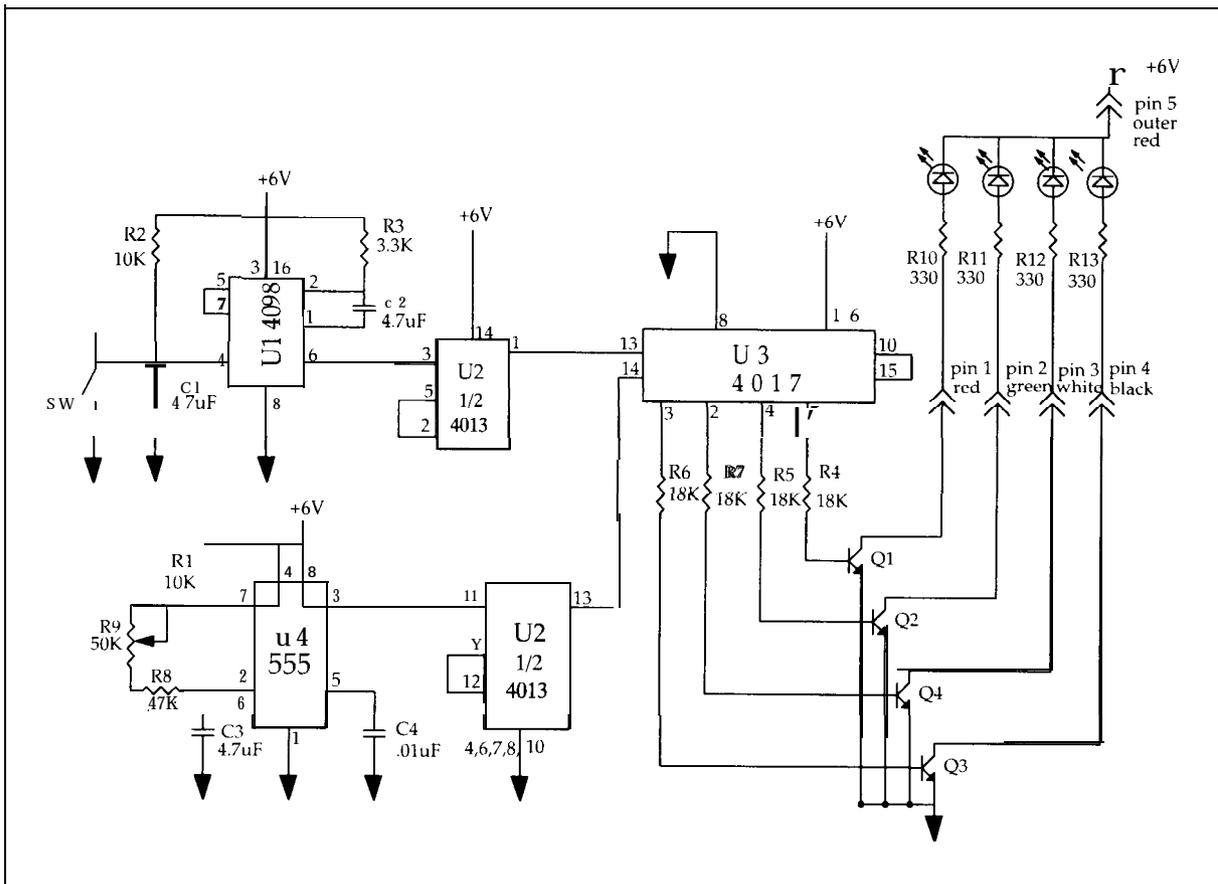
Figure 3.7. Schematic of Visual Scanner Circuitry.
