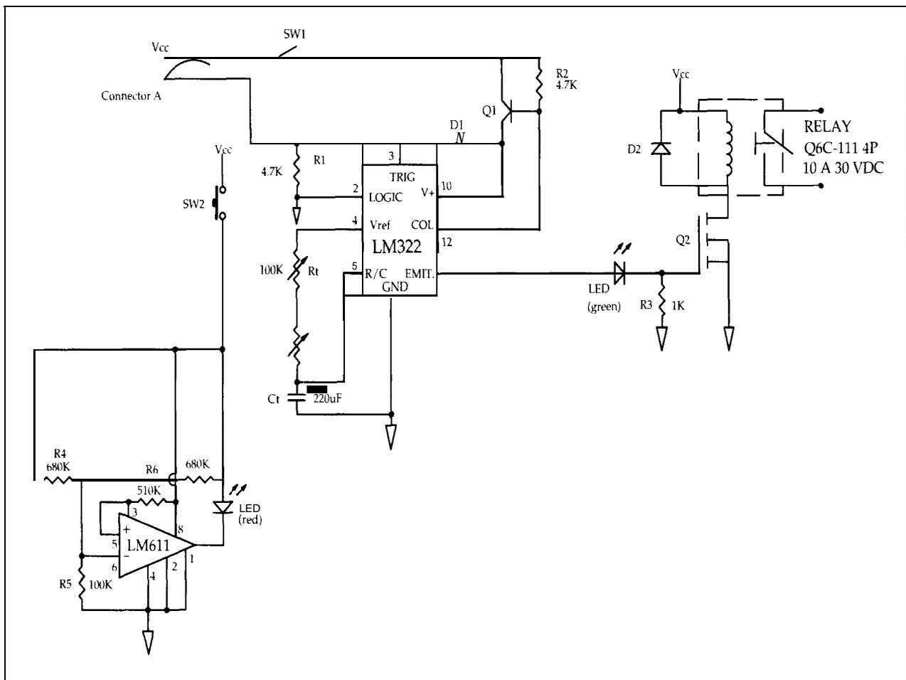
Figure 3.5. Schematic of Timer Switch circuits.
