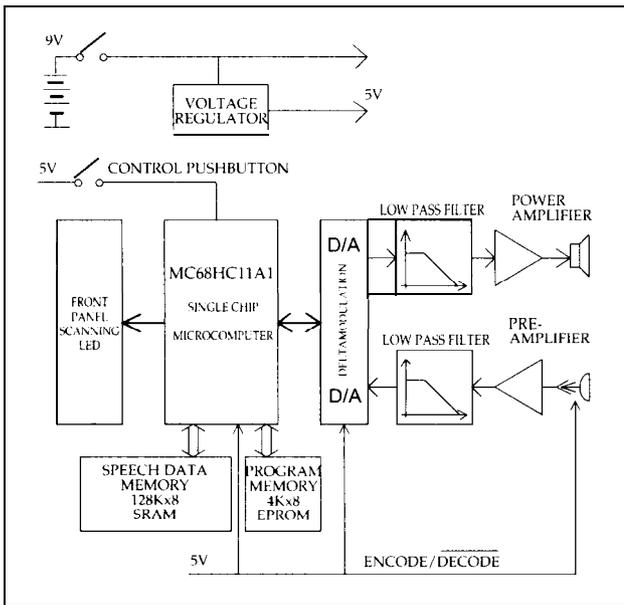
Figure 3.2. Block diagram of Speech Aid circuitry.
