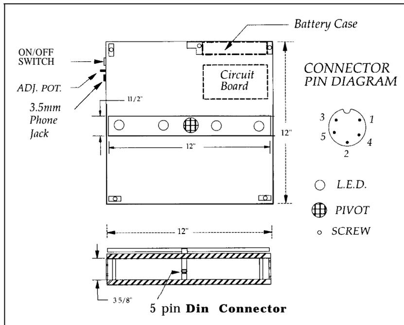
Figure 3.6 Physical drawing of Visual Scanner device.
