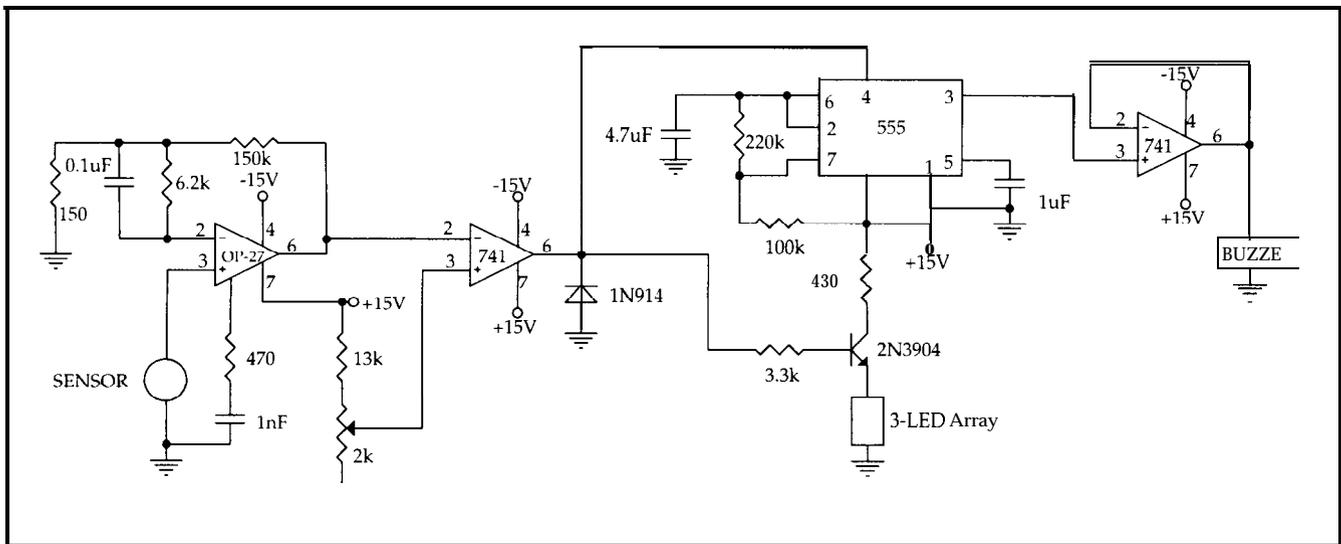
Figure 22.2. Circuit Diagram of Heat Sensor and Alarm.
