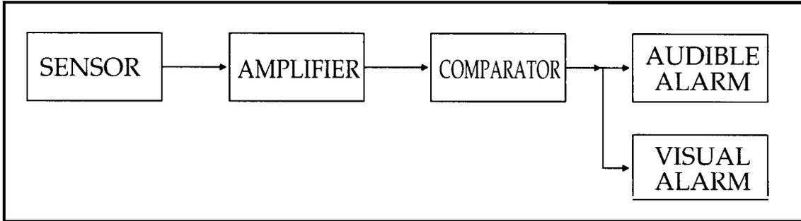
Figure 22.1. Block Diagram of Heat Sensor and Alarm.
