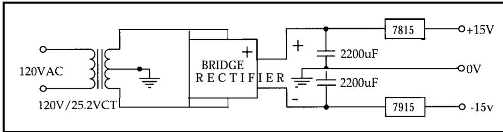
Figure 22.3. Conventional Transformer-Operated Bridge Rectifier Power Supply.
