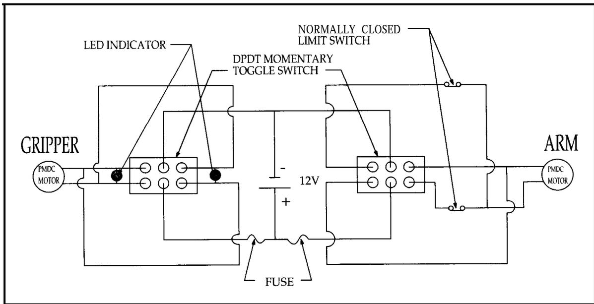
Figure 20.4. Wiring Schematic for Reacher/Gripper Device.
