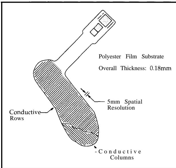
Figure 14.8. The Foot Sensor Device.
