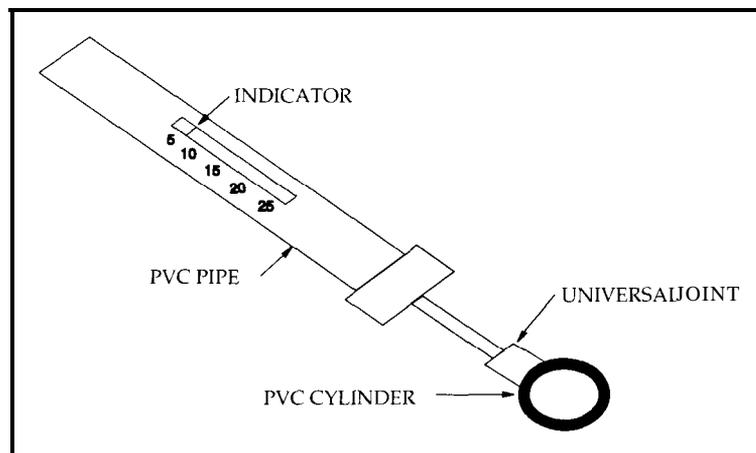
Figure 14.9. Extensometer.
