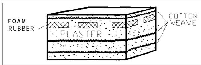
Fig. 6.3. Cross-section of Multilayered Plaster Mold.
