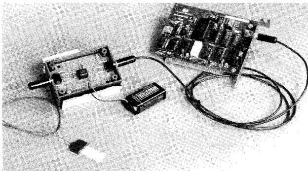
Fig. 5.5. Piezoelectric Contact Microphone for Voice Recognition.
