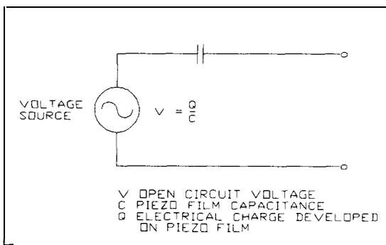
Fig. 5.6. Equivalent Circuit of Piezo Film.
