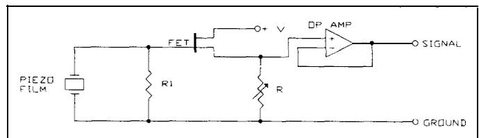
Fig. 5.8. Interface for the Intravoice VI .
