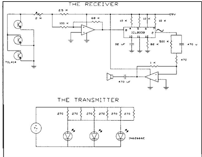
Fig. 5.2. Transmitter and Receiver Units.
