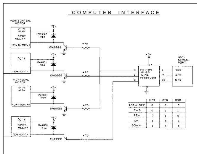
Fig. 5.1 1. Computer Interface for Turning Desk.
