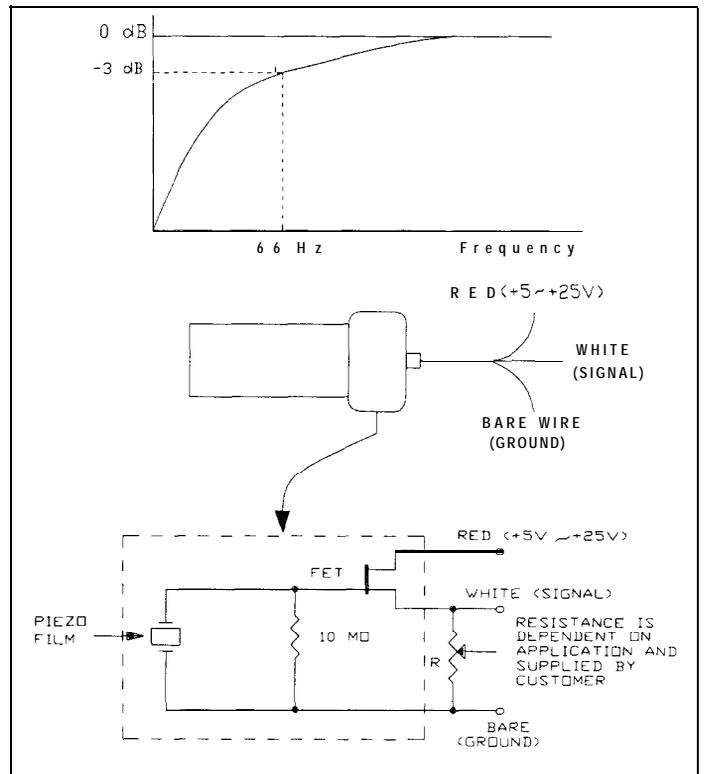
Fig. 5.7. Frequency Response of VS/FET.
