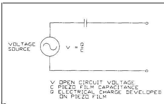
Fig. 5.6. Equivalent Circuit of Piezo Film.
