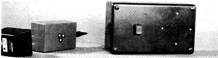
Fig. 5.1. Infrared Beacon for the Blind.
