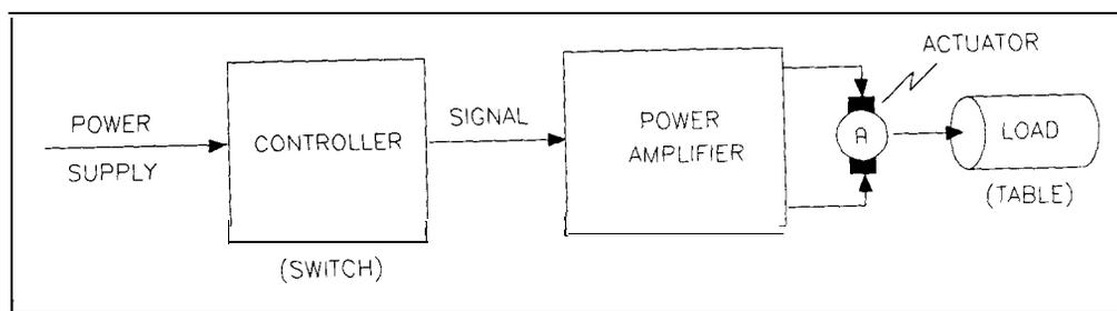
Fig. 2 1.6. Control System for Motorized Adjustable Table.
