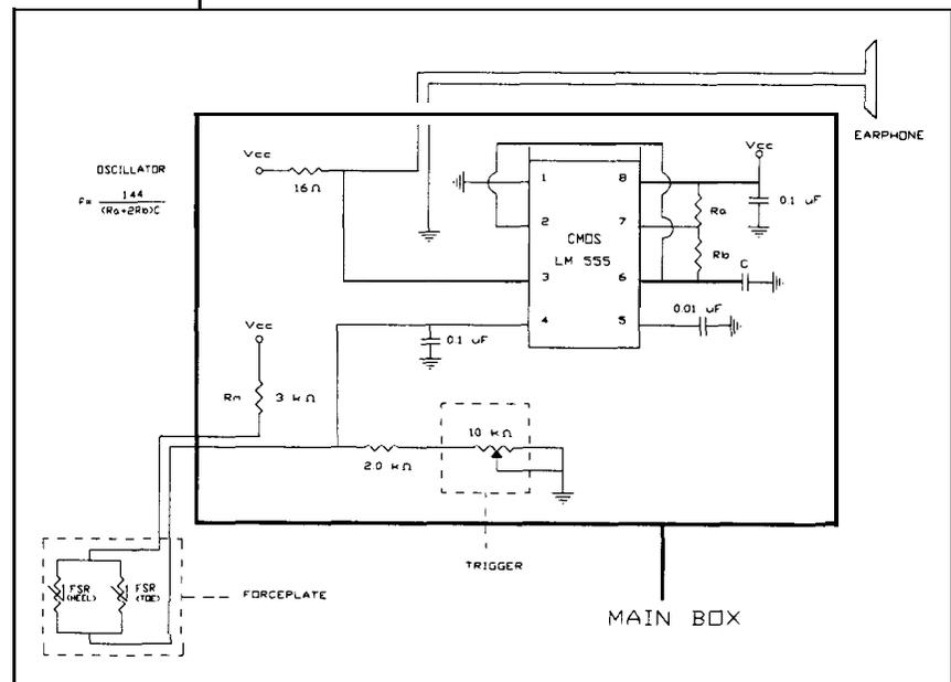
Fig. 21.4. Final Circuit Design for Gait Modification System.
