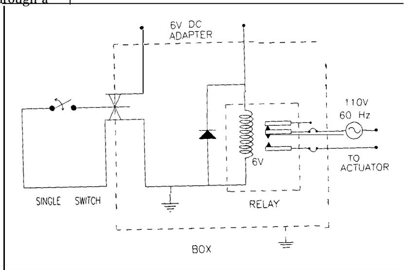
Fig. 21.7. Circuit Diagram for Motorized Adjustable Table.
