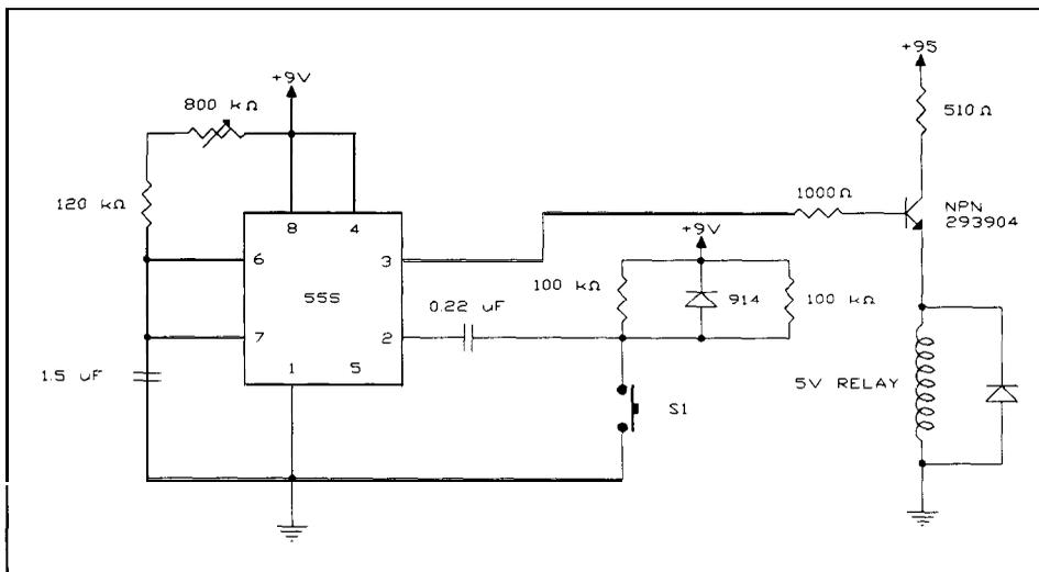
Fig. 21 .1 4. Circuit Diagram for the Electronic Timer for a Muscle Stimulator.
