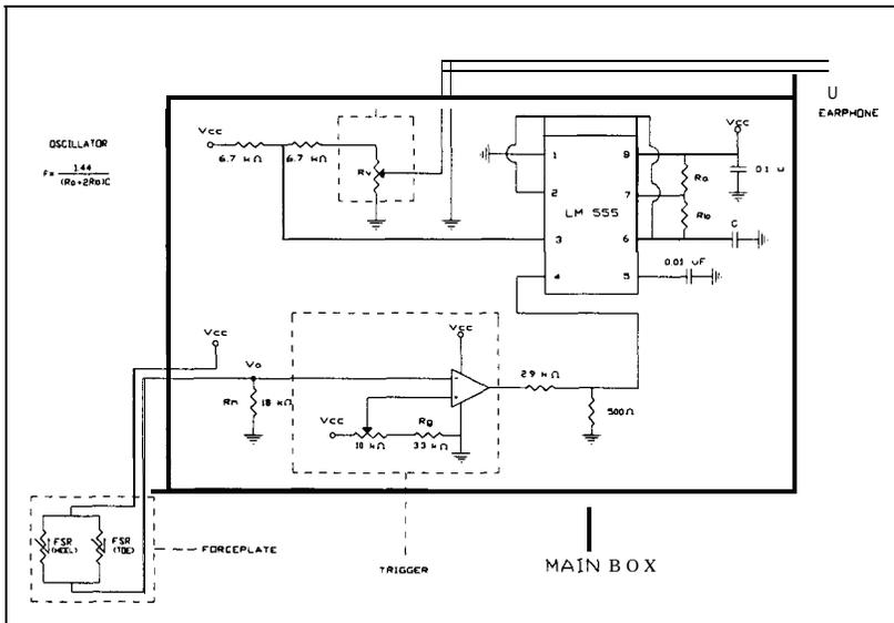
Fig. 21.3. An Improved Circuit for Gait Modification System.
