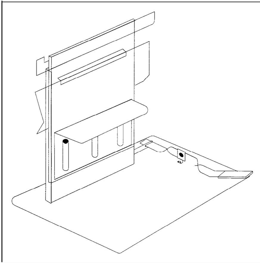
Fig. 21.9. Mechanical Drawing of the Portable Device to Highlight Individual Reading Lines.
