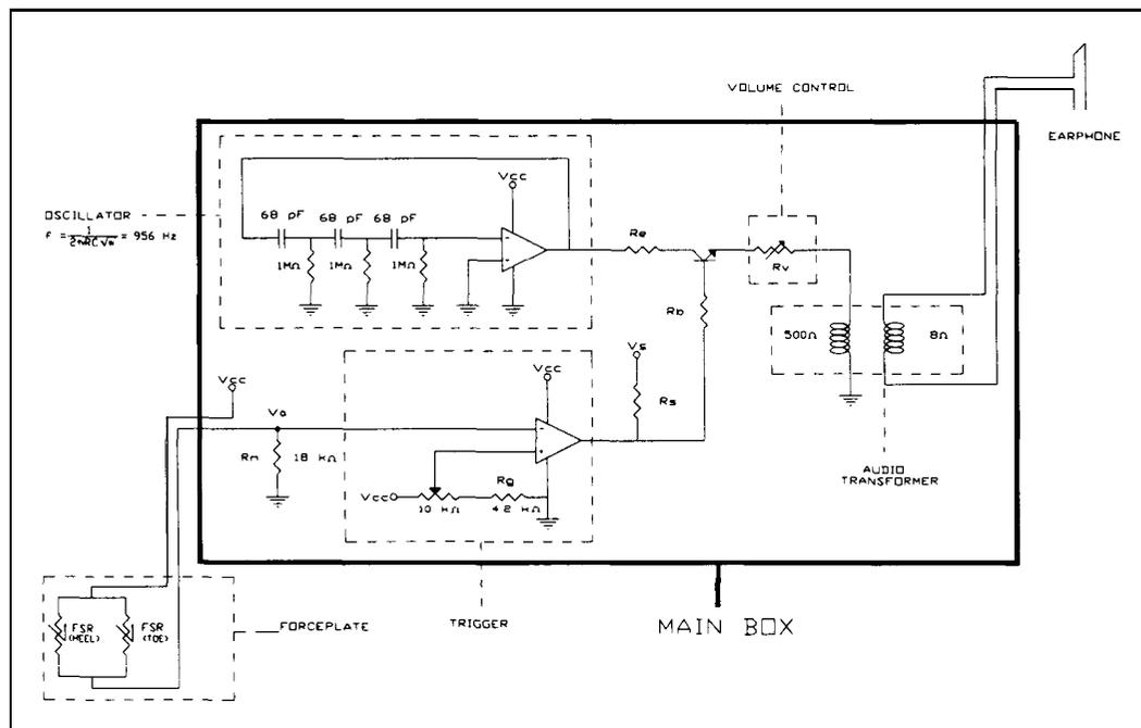
Fig. 21.2. Circuit for Gait Modification System.
