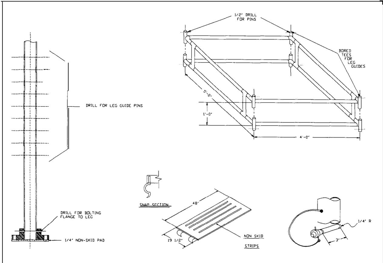
Fig. 18.7. Structure Diagram for the Hydrotherapy Platform.
