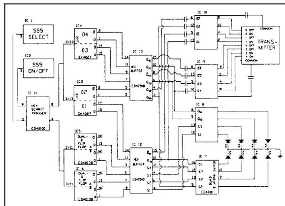
Fig. 18.5. Circuit Diagram for the Environmental Control Device.
