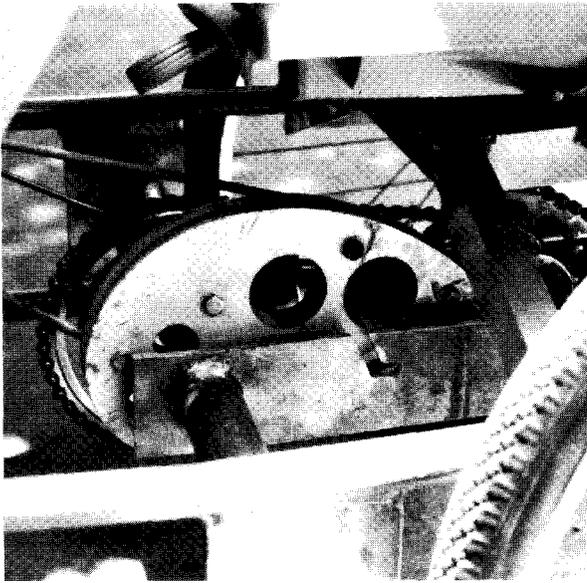
Fig. 14.2. Close-up of Hyperbolic Cam in the Drive-Train.
