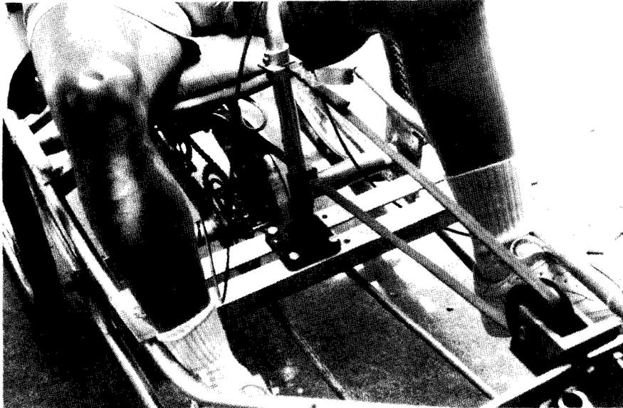
Fig. 14.3. Detail of T-bar, Strap, Cam, and 3-Speed Hub.
