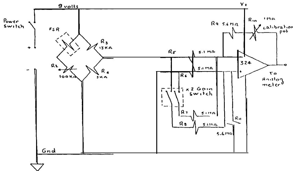
Pressure meter. circuit Diagram
